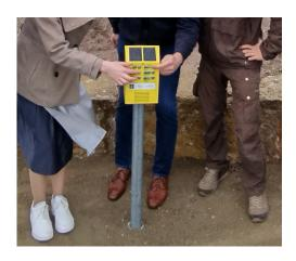
The ActiveGuide requires no connection to the electricity grid. Thanks to its hand crank, visitors can power it with muscle power alone. The SolarGuide model integrates a solar panel, ensuring sufficient energy from the skies. The speaker plays MP3 files in outstanding audio quality. The volume can be pre-set as required.
